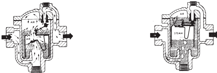
Fig. 18-1— Thermic bucket operation. At left, thermic vent is open and air “passes” through. At right, thermic vent is closed and trap operates same as a standard trap.
